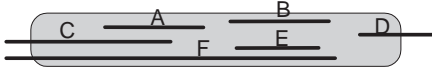
Figure 9: Illustration of Onodes/Rnodes. The shadow area is a power rail. All segments inside are Onodes. A, B and D have no parent nodes in this power rail. Thus A, B and D are URnodes. F and E have no child nodes in this power rail. They are DRnodes. A node can be both URnode and DRnode, like D.
