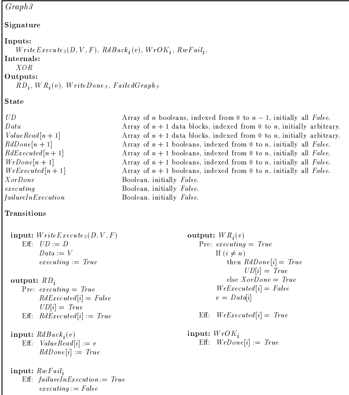
Figure 2-10: I/O Automaton for Graph 3 - Small Write
