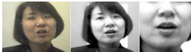
Figure 1: Face, facial part detection, and ROI extraction for an example video frame. Left-to-right: Original frame with eleven detected facial parts super-imposed; face-area enhanced frame; normalized ROI.
