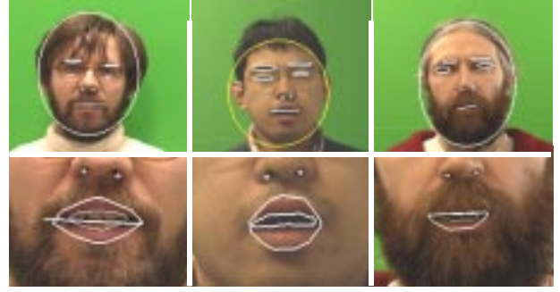
Figure 3: Examples of identified facial features (upper row) and outer and inner lip contours (lower row) for three subjects (from Parts 1 and 2 of our database).
