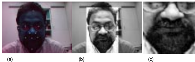
Fig. 2. Region-of-interest extraction for an example video frame in the real-time prototype: (a) Face and facial part detection, with 11 estimated facial features depicted. (b) Face-region lighting compensation. (c) Final extracted ROI, appropriately normalized.
