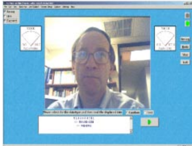
Fig. 5. The prototype graphical user interface. Two central windows depict the captured video and uttered vs. recognized text, while two meters show the resulting audio-only vs. audio-visual word error rates.
