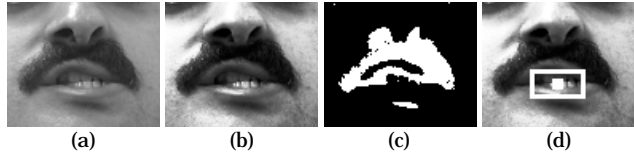
Figure 1: Visual front end: (a) Original Y-band frame; (b) histogram equalized frame; (c) thresholded frame; (d) mouth center and frame region boundary where DWT is applied.
