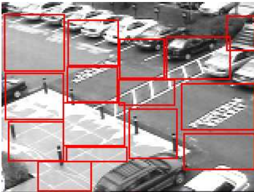
Figure 1: A master camera’s view tiled with regions of interest each tied to a bead location of a slave camera. Each slave may have such a tiling in each master view.
