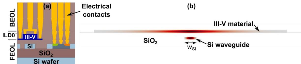
Figure 1. a) Schematic cross-section of the laser device, integrated between BEOL and FEOL of a CMOS chip. b) Simulated intensity field of the fundamental mode.
