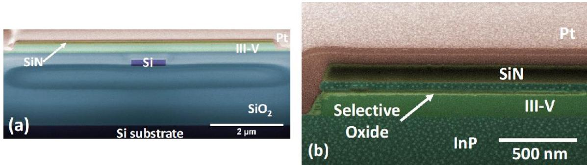
Figure 5. False-colored SEM cross-sections of a) final laser device (Si waveguide and III-V epitaxial layer stack are visible, halo in BOX originates from charging) and b) III-V epitaxial layer stack with selective lateral oxidation (only a single layer is oxidized).
