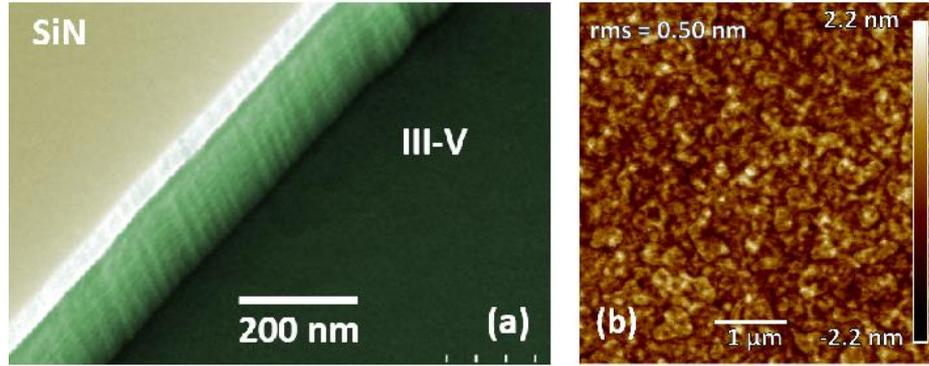
Figure 4. False-colored SEM image of the dry etched III-V stack, showing smooth sidewalls and etched surfaces. b) AFM image of the etched surface showing a roughness of 0.5 nm rms.
