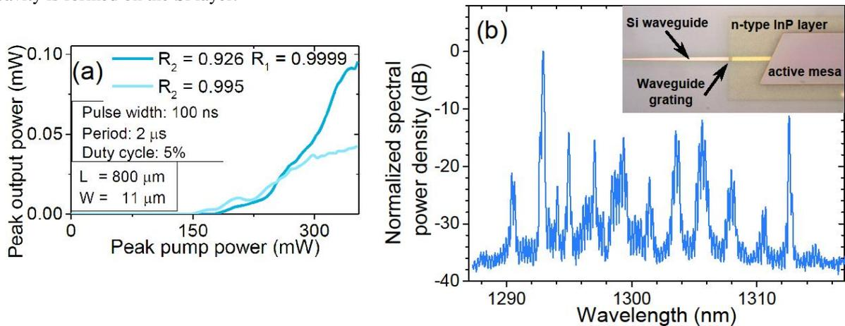
Figure 6. a) Room temperature L-I curve of two optically pumped lasers showing output power dependence of mirror reflectivity  $R_2$ . A threshold power density of  $1.7 \text{ kW cm}^{-2}$  is measured for the higher reflectivity device. b) Room temperature optical spectrum of laser device. Inset: Top-view photograph of laser device (the Si waveguide is tapered down to the bus waveguide width of 500 nm on the left).
