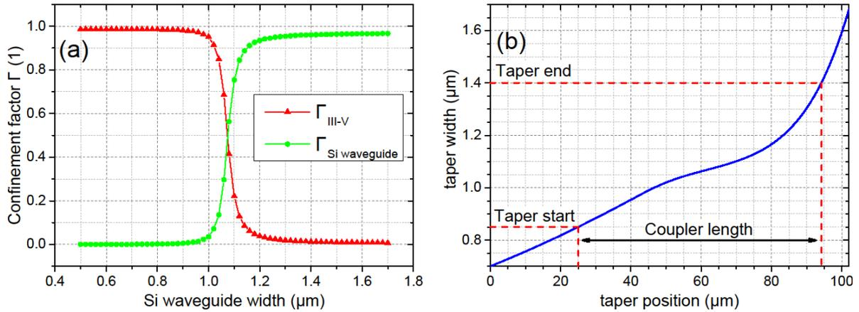
Figure 2. Design of the adiabatic coupler: a) Calculated mode overlap (confinement factor  $\Gamma$ ) versus Si waveguide width for the entire III-V stack (triangles) and the Si waveguide (circles). b) Nonlinear taper geometry for adiabatic couplers, calculated with adiabaticity criterion.
