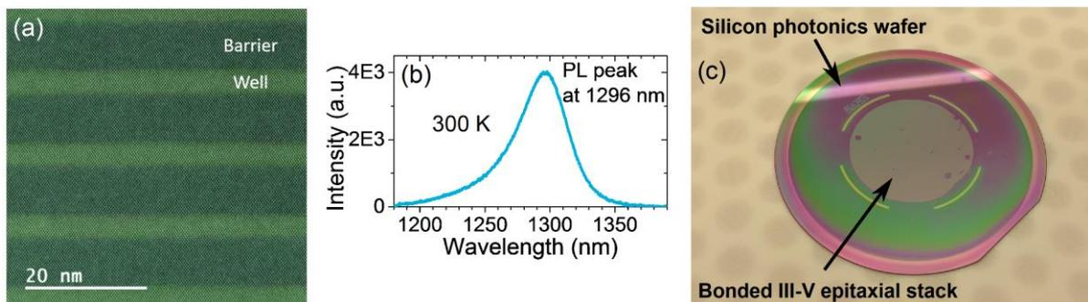
Figure 3. a) STEM image of MQW with atomically flat interfaces. b) Room temperature PL measurement of the gain material. c) Photograph of the two bonded wafers after InP substrate removal.
