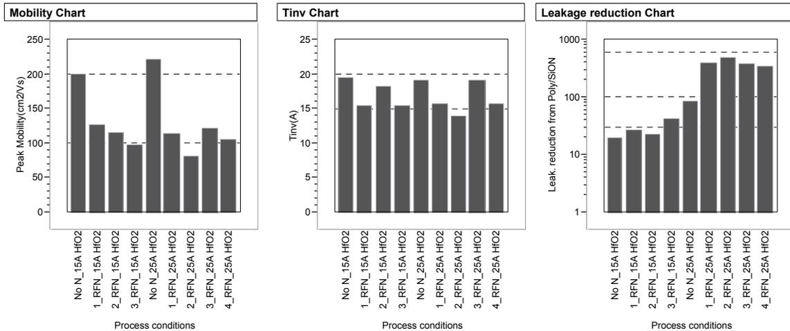
Fig. 5. Electron mobility, inversion layer thickness and leakage reduction charts of a  $W(=20\mu\text{m}) \times L(=5\mu\text{m})$  N-FET as a function of various RF nitridation processes of interfacial layer only. The gate stack was annealed at 1000 °C. Data are shown for two different  $\text{HfO}_2$  thicknesses, 1.5 and 2.5 nm.
