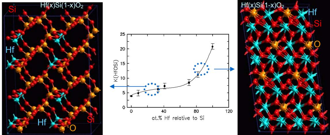
Fig. 2. Hf silicate structures which may form after a high temperature annealing of W/HfO<sub>2</sub>/SiO<sub>2</sub>. Center is a plot of silicate dielectric constant as a function of Hf at. % relative to Si<sup>11</sup>. At low Hf content the silicate structure is a SiO<sub>2</sub> matrix with Hf embedded (left). At high Hf content the silicate structure is a HfO<sub>2</sub> matrix with Si embedded (right).
