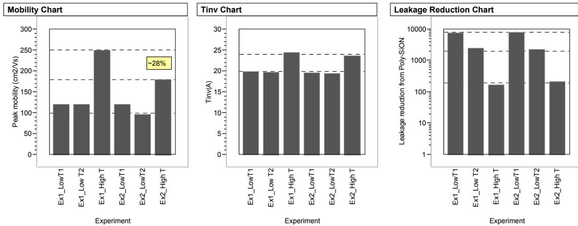
Fig. 3. Electron mobility, inversion layer thickness and leakage reduction charts of a W(=20 $\mu$ m) x L(=5 $\mu$ m) N-FET as a function of annealing temperature; LowT1~500 °C, High T~1000 °C. Gate stack is W/HfO<sub>2</sub>/SiON. In Ex2 the SiON layer was spike annealed at 1100 °C, in Ex1 the SiON was not spike annealed.
