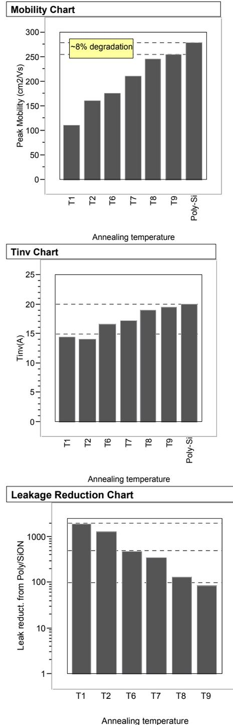
Fig. 1. Electron mobility, inversion layer thickness and leakage reduction charts of a W(=20 $\mu$ m) x L(=5 $\mu$ m) N-FET as a function of annealing temperature; T1~400 °C, T9~1000 °C. Gate stack is W/HfO<sub>2</sub>/SiO<sub>2</sub>.
