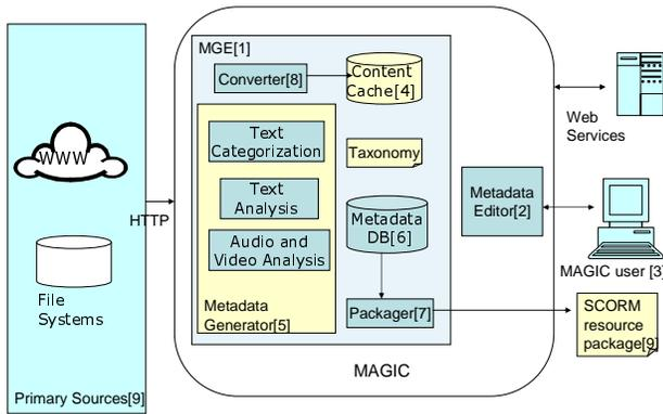
Figure 1. High-level MAGIC system architecture.
